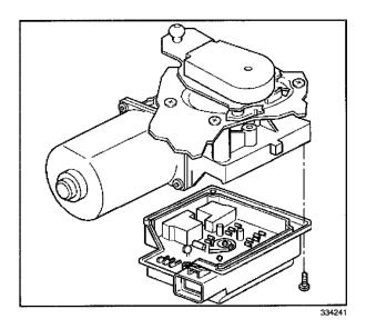
1. Position the wiper motor cover to the wiper motor.
