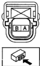
Fig. 19: Identifying PCV Valve Heater Control Connector Terminals Courtesy of MAZDA MOTORS CORP.
