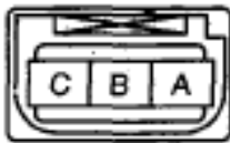
FUEL TANK PRESSURE SENSOR WIRING HARNESS-SIDE CONNECTOR
