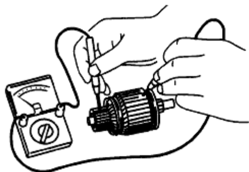
Fig. 8: Checking Continuity Between Commutator And Core At Each Segment Using Tester
