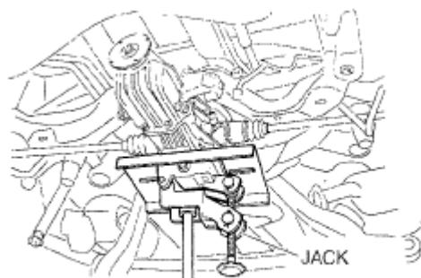
Fig. 7: Supporting Rear Differential Courtesy of MAZDA MOTORS CORP.
