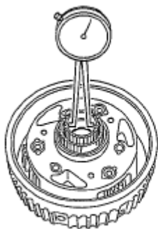
Fig. 167: Measuring Inner Diameter Of Rear Planetary Gear Bushings Courtesy of MAZDA MOTORS CORP.
