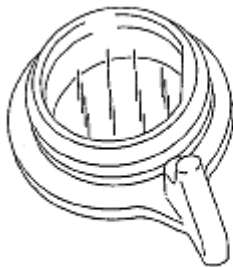
Fig. 286: Inspecting Condition Of Connector Pin Of Coupler Component (Foreign Material, Bent/Broken Pins) And O-Ring Courtesy of MAZDA MOTORS CORP.
