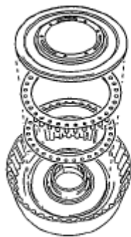
Fig. 100: Identifying Retainer, Return Spring And Clutch Balancer Courtesy of MAZDA MOTORS CORP.
