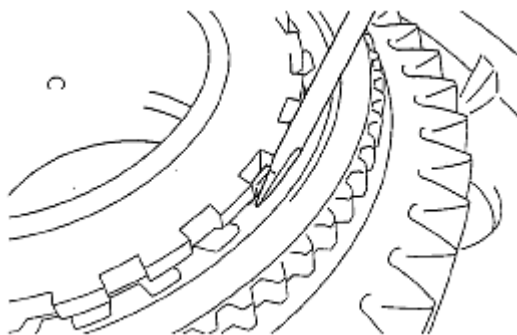
Fig. 157: Crimping Down Washer Courtesy of MAZDA MOTORS CORP.
