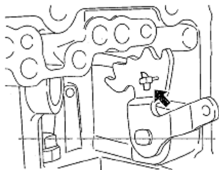
Fig. 242: Locating Parking Rod Of Manual Valve Lever Courtesy of MAZDA MOTORS CORP.
