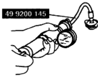
Fig. 9: Applying Pressure With Radiator Cap Tester Courtesy of MAZDA MOTORS CORP.
