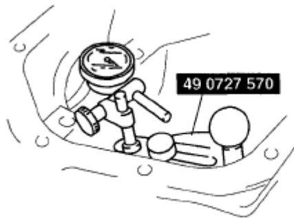
Fig. 40: Measuring Probe Of Dial Indicator Courtesy of MAZDA MOTORS CORP.
