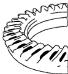
Fig. 49: Inspecting Tooth Contacts Courtesy of MAZDA MOTORS CORP.
