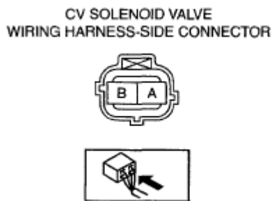
Fig. 10: Identifying CV Solenoid Valve Wiring Harness-Side Connector Courtesy of MAZDA MOTORS CORP.
