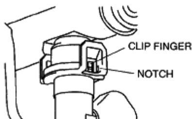
Fig. 44: Identifying Clip Fingers & Notch
