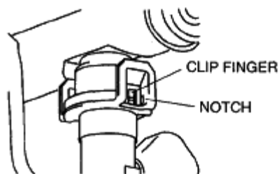
Fig. 44: Identifying Clip Fingers & Notch
