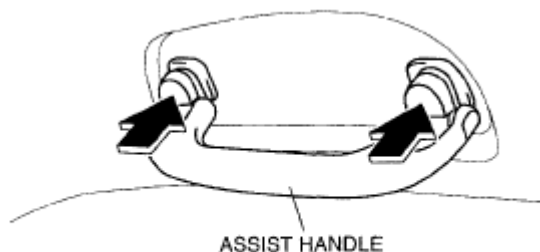
Fig. 79: Pushing Assist Handle Courtesy of MAZDA MOTORS CORP.
