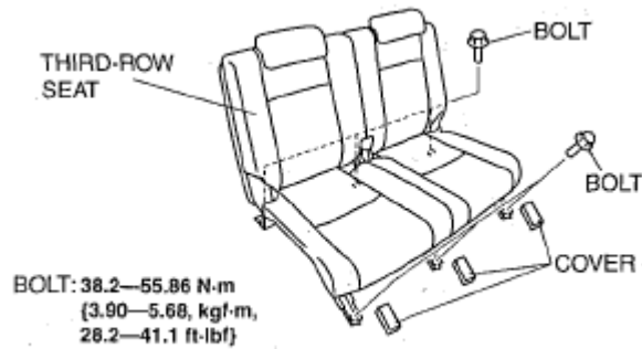
Fig. 41: Identifying Third-Row Seat, Bolt & Torque Specifications Courtesy of MAZDA MOTORS CORP.
