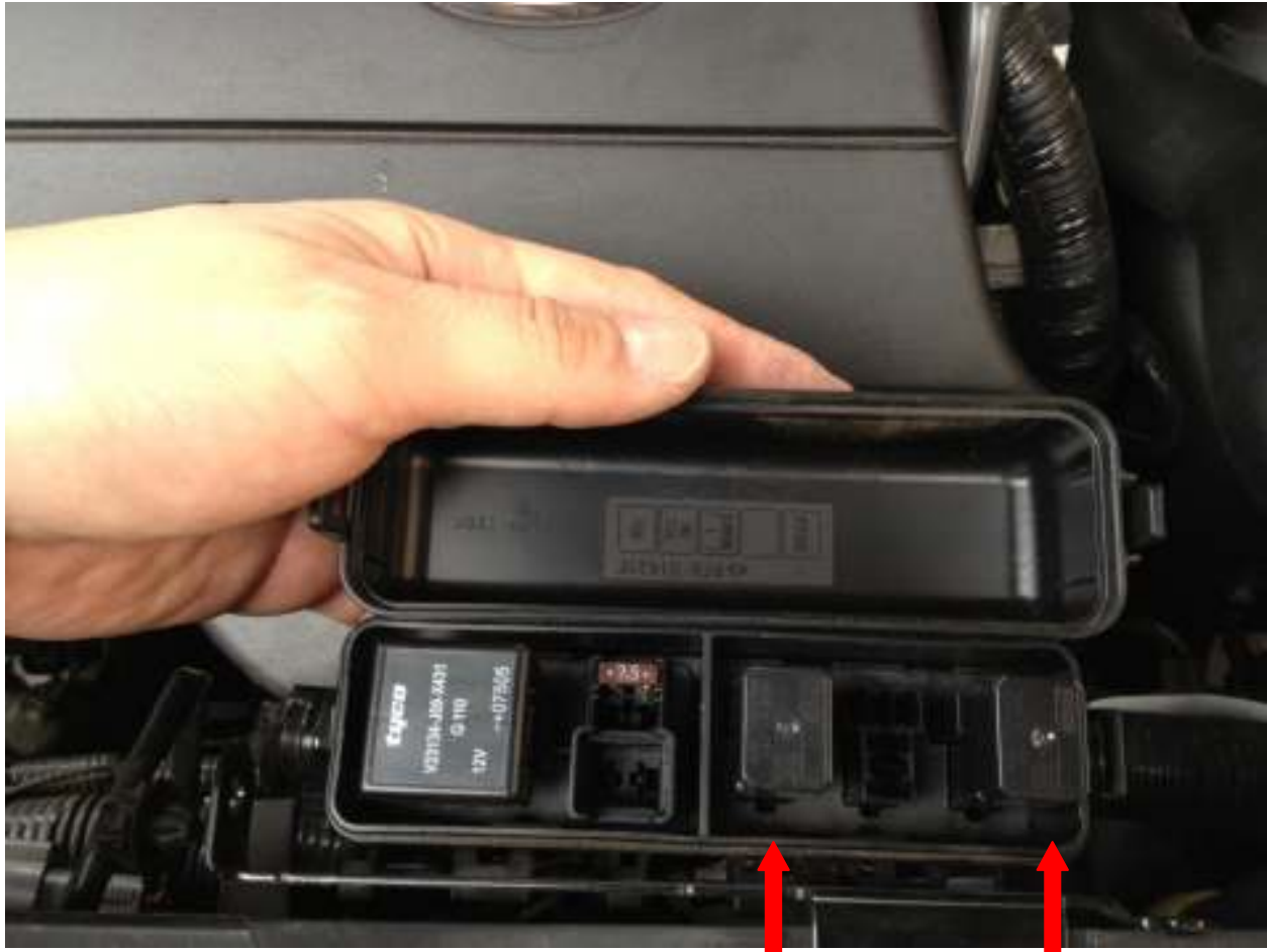
Seat warmer relay on left. Fog light relay on right
