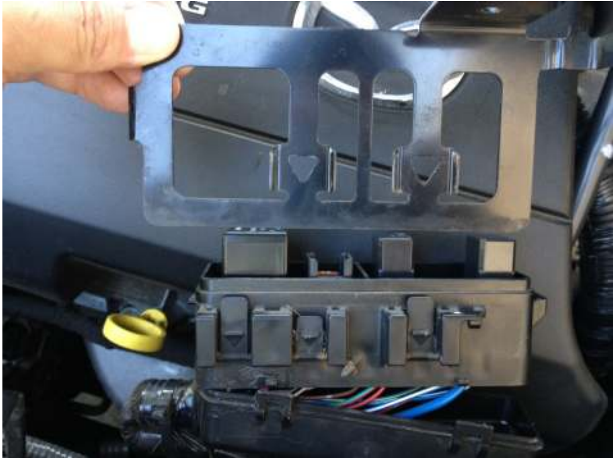
Removed, leaving the relay box clearly visible
