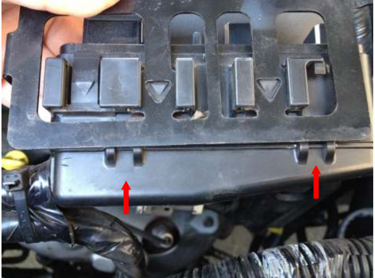
The bottom piece of the relay box must be removed. Two tabs in the back
