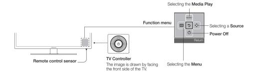
Exits the menu when pressing the controller more than 1 second. Nhen selecting the function by moving the controller to the up/down/left/right directions, be sure not to press the controller. If you press it first, you cannot operate it to move the up/down/left/right directions.
