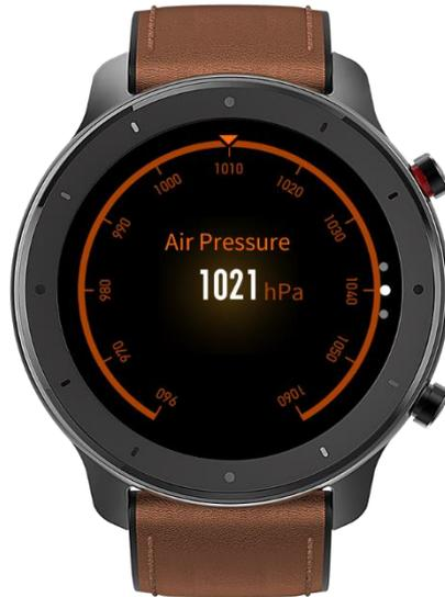
Sliding up on the air pressure page can enable you to enter the altitude page. The altitude requires double calibration of watch barometer and GPS. If you want more accurate altitude data, try to get the satellite positioning in an open area as soon as possible.
